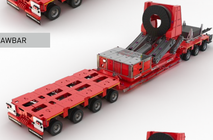
COMBINATION WITH MODULAR SELFPROPELLED VEHICLE
