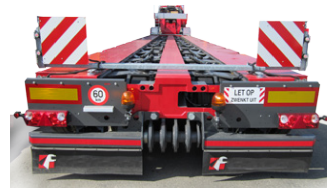
Lighting with underrun protection and warning boards
