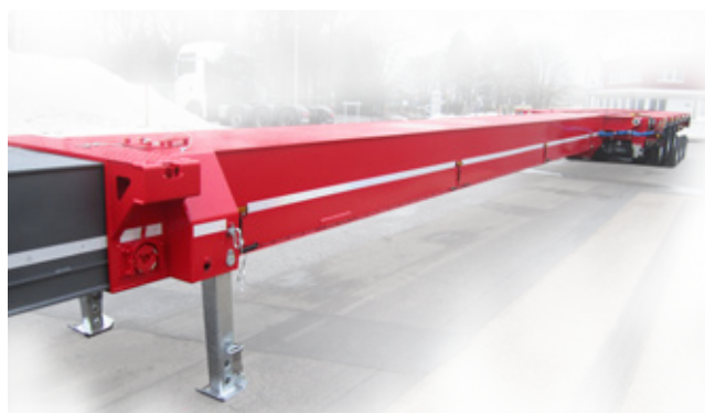
Extendable spacer beam for modular trailers
