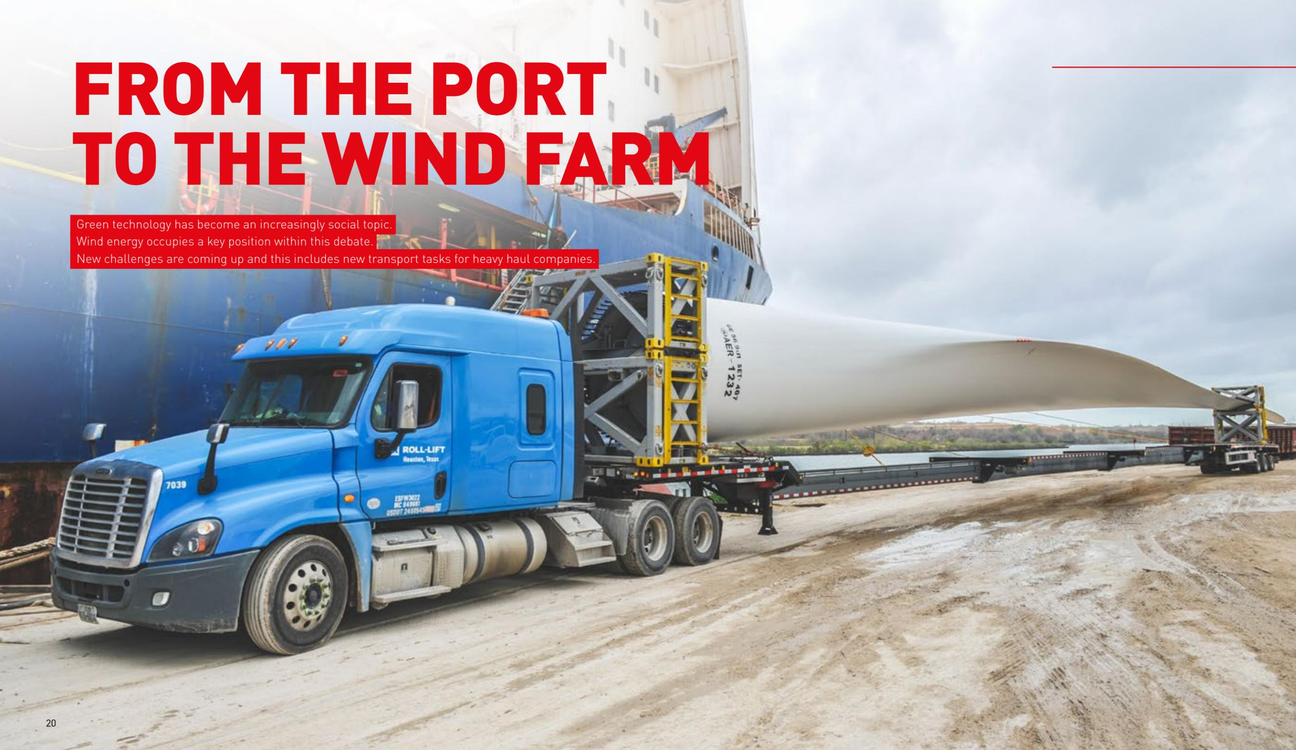
Blue goes green! A short pun describing how Roll-Lift USA, Inc. from Dayton, Texas takes on the job of moving a new delivery of wind turbine blades. A mission made for their four 3-axle TeleMAX trailers with trucks in typical blue. With their four extensions, these trailers reach a total open length of 200', composed of 176' deck length and a 24' non-load bearing pull-out to allow for a longer overhang.
