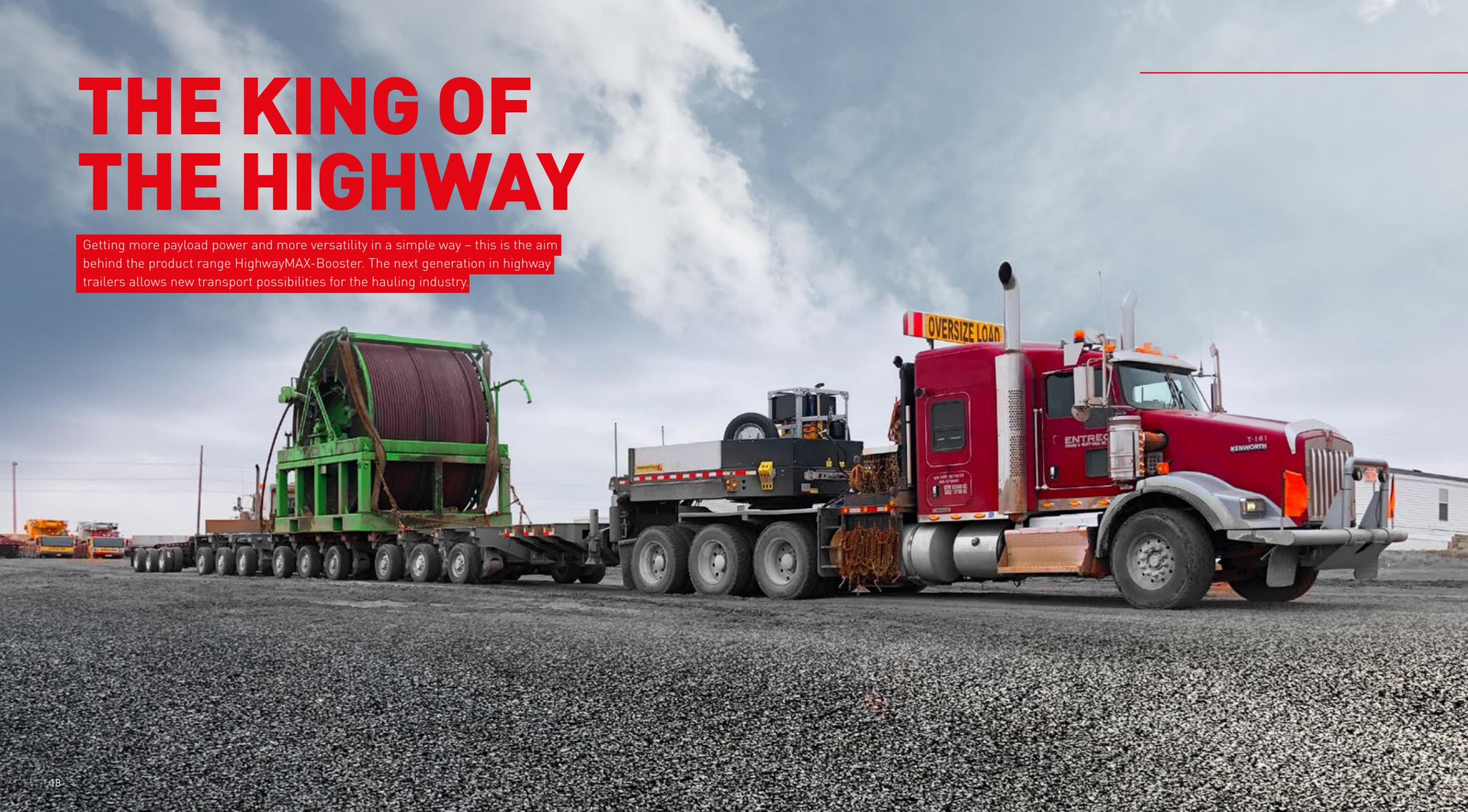
The principle behind it is as simple as ingenious. A 3-axle chassis and self-tracking pivot design is coupled to the back of the trailer when heavy load needs to be moved. By using the booster, the number of axles is increased over which the weight is distributed, thanks to well thought-out pressure transfer. This process creates an overall increase in payload capacity. A 9+3 axle trailer/booster combination adds up to a legal payload of around 205,000 lbs at 20,000 lbs per axle.
